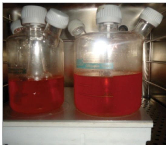
Fig. 1. MDCK-SIAT1 cell growth on Cytodex-1 microcarriers in spinner-flask cultivation
