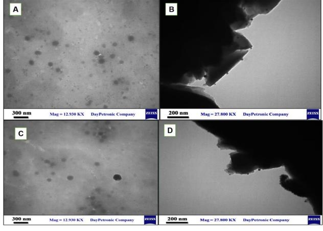
**Fig. 3.** Transmission electron microscope and Scanning electron microscopy (SEM) images of chitosan NP (**A and B**) and influenza antigen loaded onto chitosan (**C and D**) showing morphological features of the NP in the ratio of 1:2 chitosan/TPP. The scale bars are presented in each panel.
