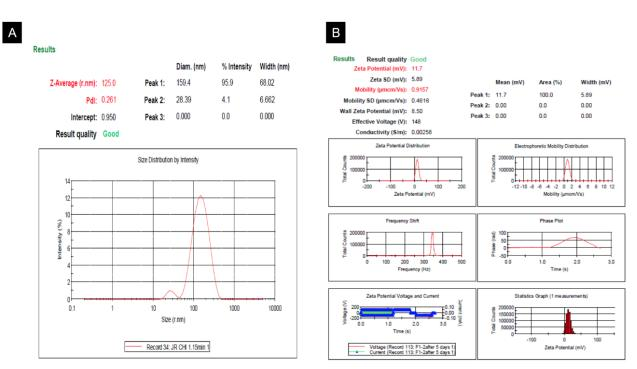
Fig. 1. (A) The size distribution of the NPs. (B) Surface charge of chitosan in the ratio of 1:2 chitosan/TPP.
