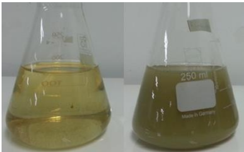
Fig. 1. Right: A flask containing AgNPs, 1 min after adding the anise extract. Left: Complete reduction, after 96 h of adding the anise extract
