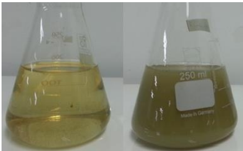
Fig. 1. Right: A flask containing AgNPs, 1 min after adding the anise extract. Left: Complete reduction, after 96 h of adding the anise extract
