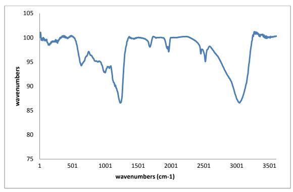
Fig. 5. FTIR spectra of the powdered AgNPs after the reduction
