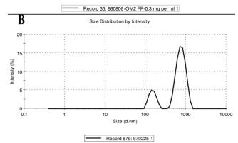
**Fig.3.** A) Size distribution report by intensity of EVs from ultracentrifugation method. B) Size distribution report by intensity of EVs from PEG-based method.
